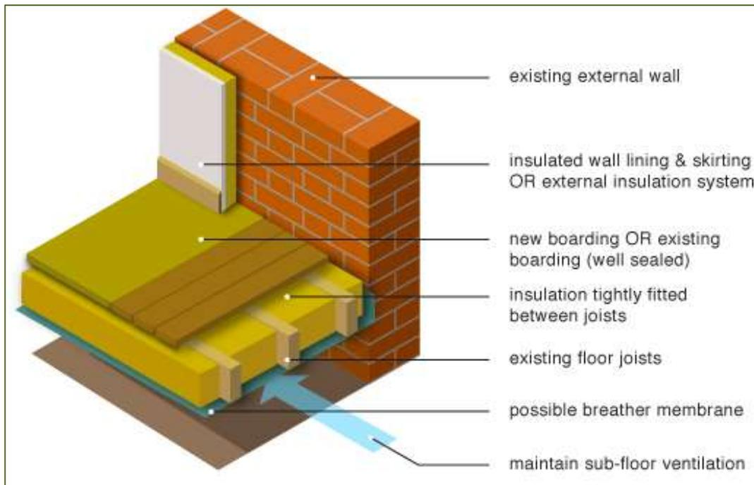
General layout of underfloor insulation for suspended timber floors
