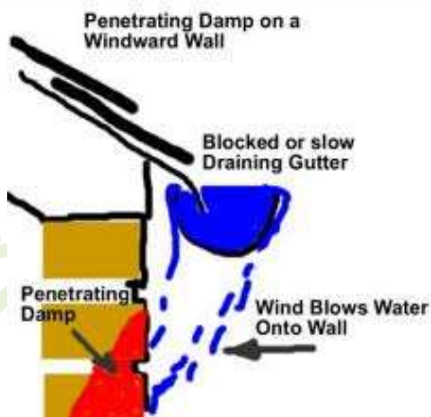
Examples of penetrating damp and rising damp mechanisms
