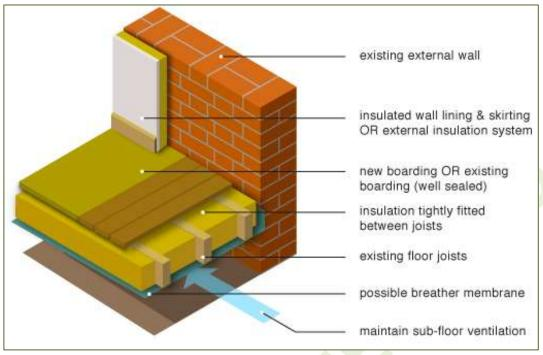
General layout of underfloor insulation for suspended timber floors Image courtesy of: <u>http://www.greenspec.co.uk/building-design/ground-floor-insulation/</u>
